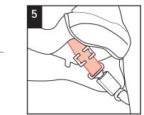
Rebuckle belt. Lap belt portion should now be tight. If not, remove locking clip and repeat all steps.
